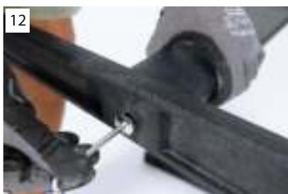
Place the crossbeam in its designated area (11) and fix it with two studs (1 per side) with the help of the Allen key nr. 6 (12). Finish by tightening all the studs well. Repeat all the operations for the other leg and turn the football table upside down.
