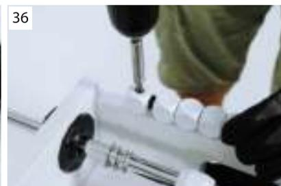
Assemble the score markers (34). Place the score marker on the lateral panel side keeping it in the middle (3.5 cm per side) (35). Insert the screws with the help of an electric screwdriver (36). Repeat the same operation on the other side.
