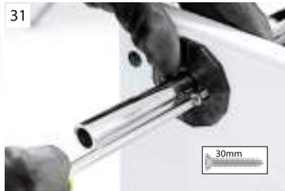
Make sure they are well wedged (30) and fix them with two screws (31). Repeat these steps for all the bearings.
